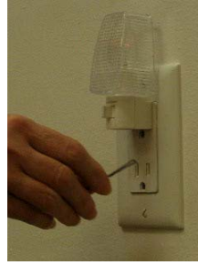
Before the Hairpin can be inserted in the outlet the power automatically turns off
